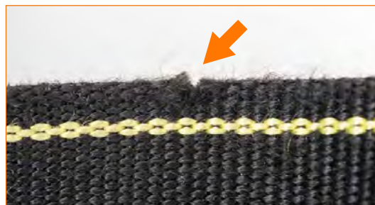
Strap with small tear on external edge.
