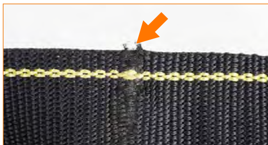
Strap has been crushed.
