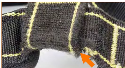
Straps very worn where they join.
